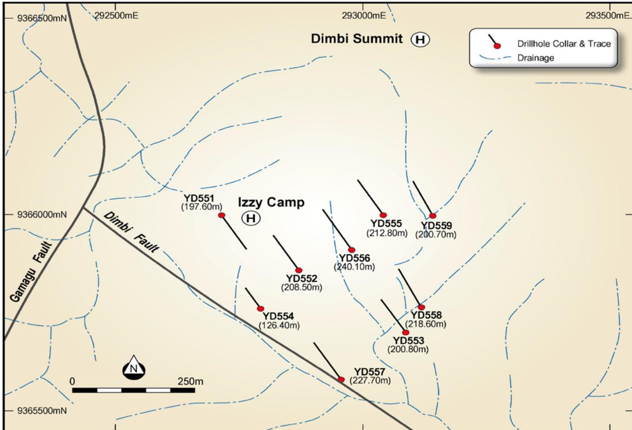
Collar coordinates were determined by hand-held GPS units and are accurate to within +/- 8m of the true location as established by GPS accuracy checks against known positions. Collars are to be re-surveyed at a later date using high precision GPS survey methods.
